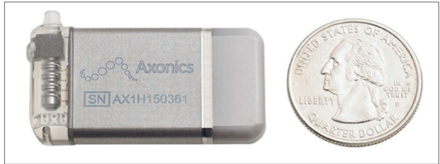
Figure 2. Size of the Axonics rechargeable neurostimulator compared to a United States quarter.
