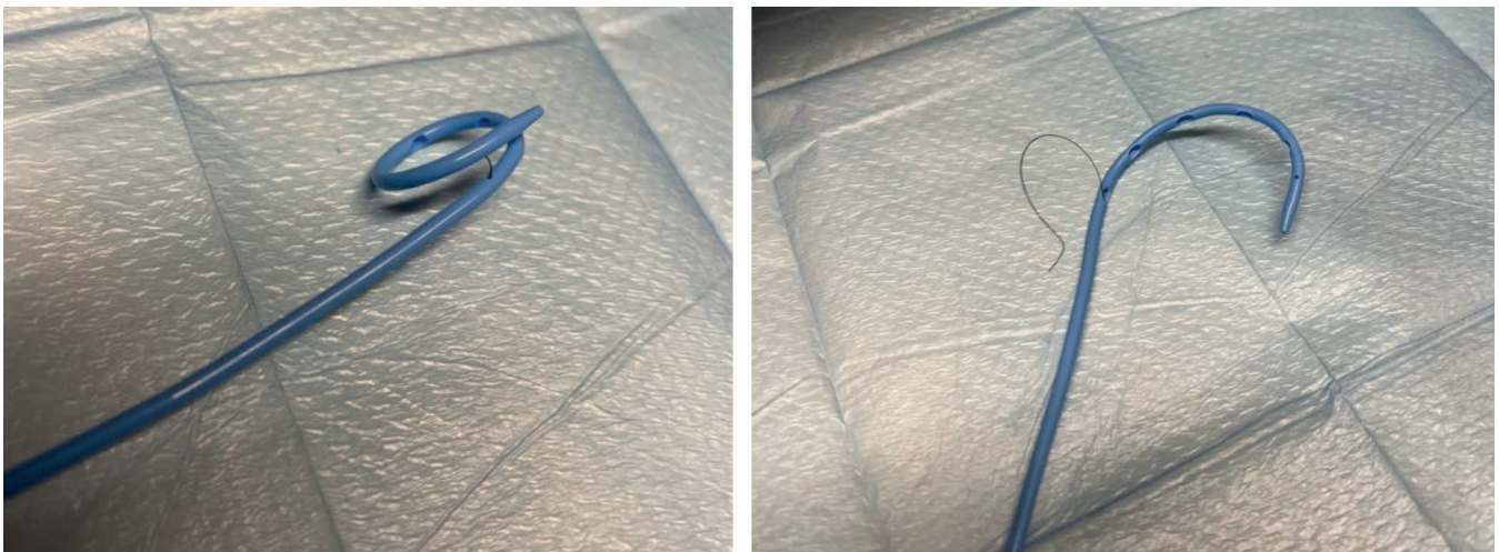
Figure 2: Normal pigtail mechanism (left) and failure allowing uncurling of the coil (right).
